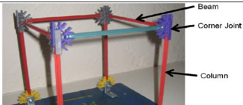
This is a generic 1st story for a knex structure. The vertical rods make up the columns and the horizontal rods make up the beams (and the floors) of the structure. The corner joints connect the beams and columns together and leave room for joints.
